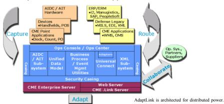
**AIDC** /**AIT support:** AdaptLink incorporate native support for technologies such as Radio Frequency Identification (RFID), barcodes, and more.
